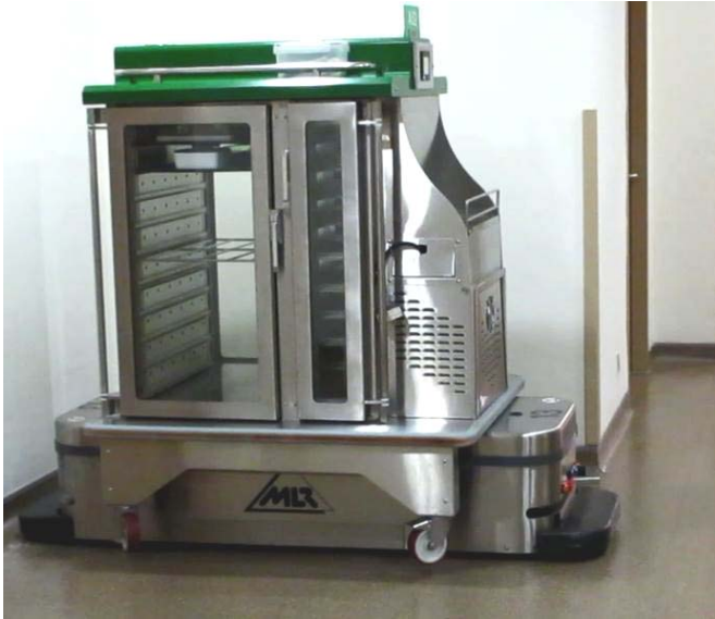
Figure13: Typical AGV with a supply trolley
