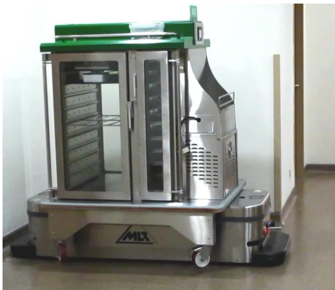
Figure15: Typical AGV with a supply trolley
