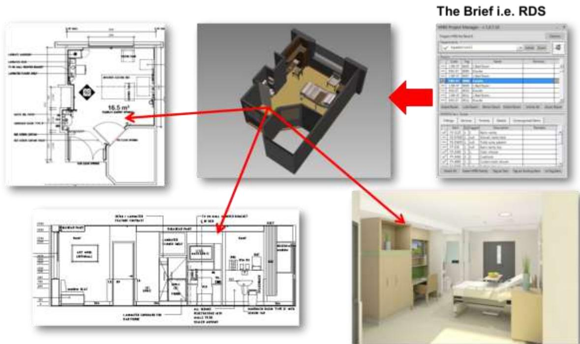
Figure 12: Room Data Sheet & Room Layout Sheet
